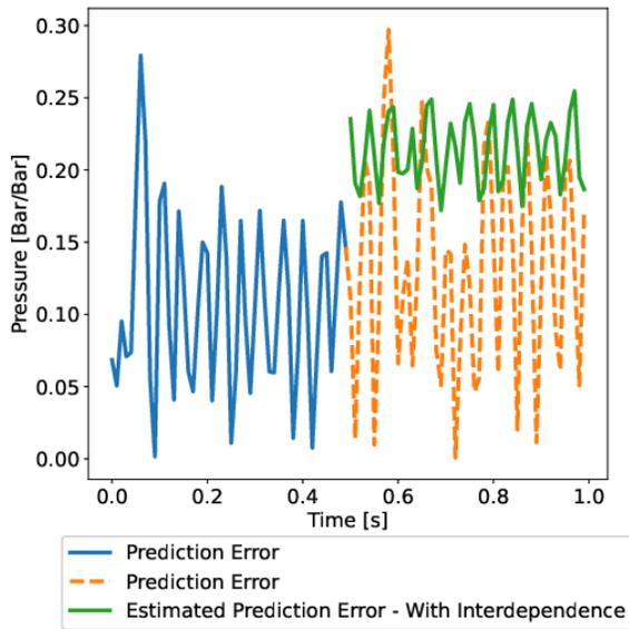
**Figure 11: Prediction error and estimated prediction error for the PS6 sensor before and after its measurements are replaced by predictions. The measurements from PS6 to be replaced by predictions at  $t = 0.5s$ , leading to a recurrent interdependence between the predictions for PS6.**
