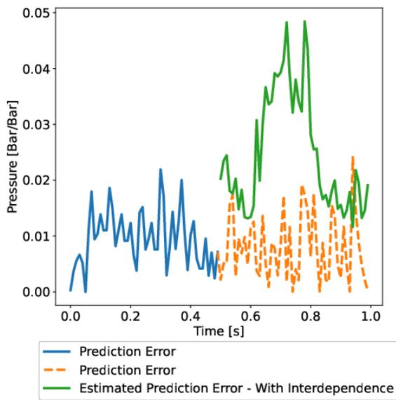
**Figure 5:** Prediction error and estimated prediction error for the PS1 sensor before and after measurements from the MPW sensor are replaced by predictions. The measurements from MPW start to be replaced by predictions at  $t = 0.5s$ , leading to interdependence between the predictions for PS1 and MPW.
