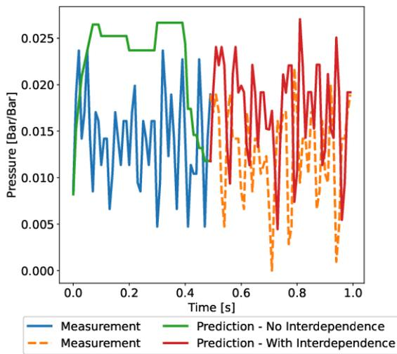
**Figure 4:** Measurements and predictions for the PS1 sensor before and after measurements from the MPW sensor are replaced by predictions. The measurements from MPW start to be replaced by predictions at  $t = 0.5s$ , leading to interdependence between the predictions for PS1 and MPW.
