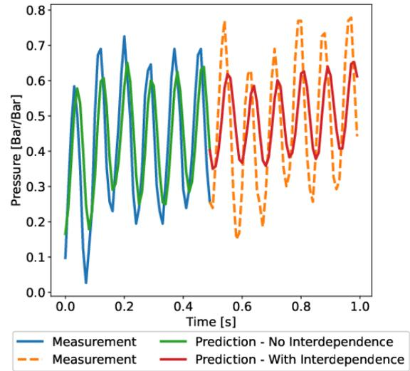
**Figure 10: Measurements and predictions for the PS6 sensor before and after its measurements are replaced by predictions. The measurements from PS6 to be replaced by predictions at  $t = 0.5s$ , leading to a recurrent interdependence between the predictions for PS6.**
