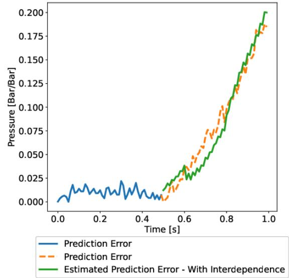
**Figure 9: Prediction error and estimated prediction error for the PS1 sensor before and after measurements from the MPW sensor are replaced by predictions. The measurements from PS1 and MPW start to be replaced by predictions at  $t = 0.5s$ , leading to interdependence between the predictions for PS1 and MPW.**
