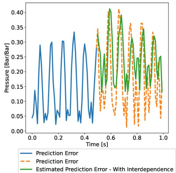
**Figure 7:** Prediction error and estimated prediction error for the PS5 sensor before and after measurements from both PS5 and PS6 sensor are replaced by predictions. The measurements from PS5 and PS6 start to be replaced by predictions at  $t = 0.5s$ , leading to interdependence between the predictions for PS5 and PS6.
