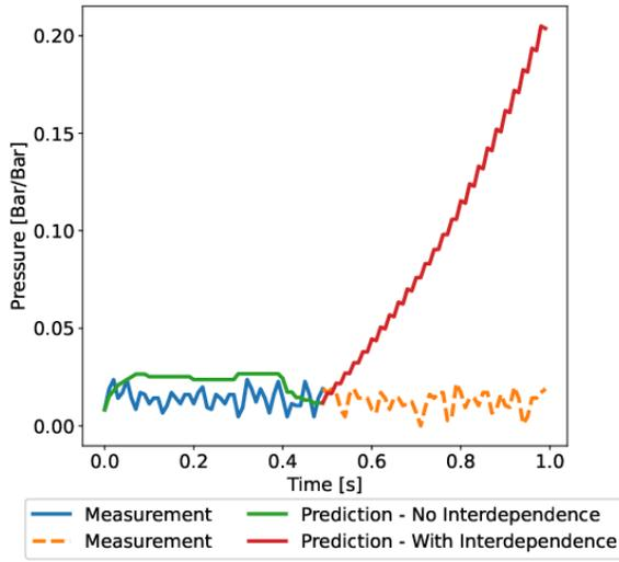
**Figure 8: Measurements and predictions for the PS1 sensor before and after measurements from both PS1 and MPW sensor are replaced by predictions. The measurements from PS1 and MPW start to be replaced by predictions at  $t = 0.5s$ , leading to interdependence between the predictions for PS1 and MPW.**
