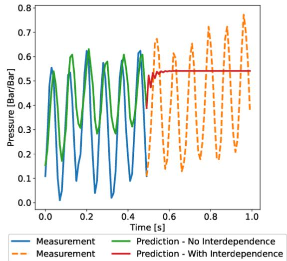
**Figure 6:** Measurements and predictions for the PS5 sensor before and after measurements from both PS5 and PS6 sensor are replaced by predictions. The measurements from PS5 and PS6 start to be replaced by predictions at  $t = 0.5s$ , leading to interdependence between the predictions for PS5 and PS6.
