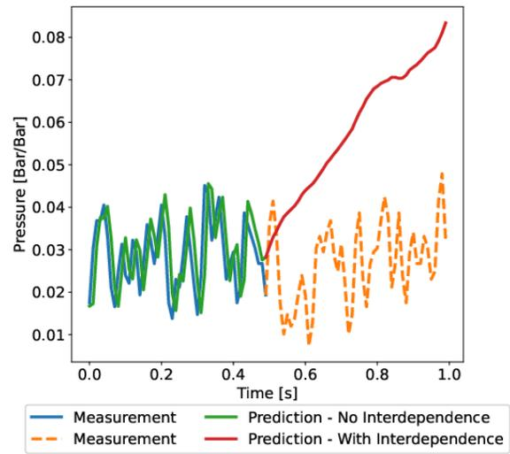
**Figure 12: Measurements and predictions for the PS2 sensor before and after its measurements are replaced by predictions. The measurements from PS2 to be replaced by predictions at  $t = 0.5s$ , leading to a recurrent interdependence between the predictions for PS2.**
