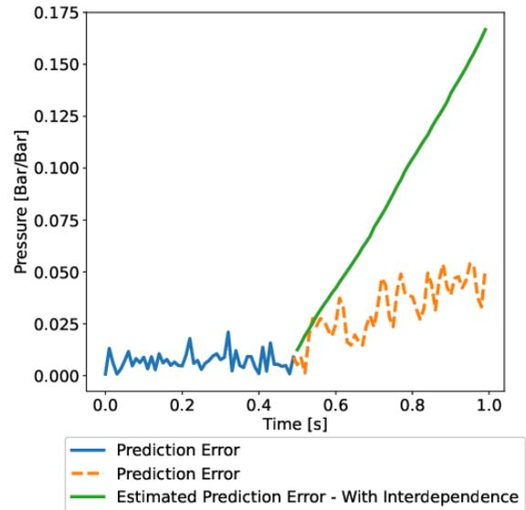
**Figure 13: Prediction error and estimated prediction error for the PS2 sensor before and after its measurements are replaced by predictions. The measurements from PS2 to be replaced by predictions at  $t = 0.5s$ , leading to a recurrent interdependence between the predictions for PS2.**
