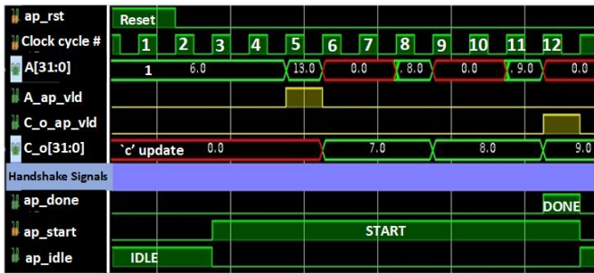
Figure 4: Waveform presenting temporal changes in RTL signals of sample function: func_foo .
