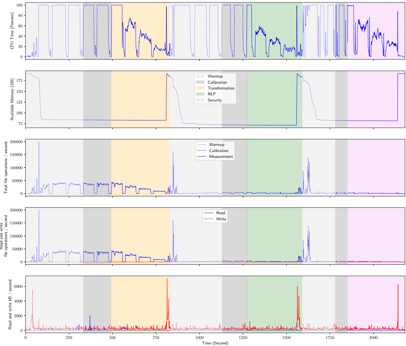
Figure 5: Preliminary measurements of CPU time, available memory, file operations, and disk data rates on a SPECpowerNext Wiki workload run. Measurement phases with four load levels, 100%, 75%, 50%, and 25%, are highlighted for each of the three worklets.
