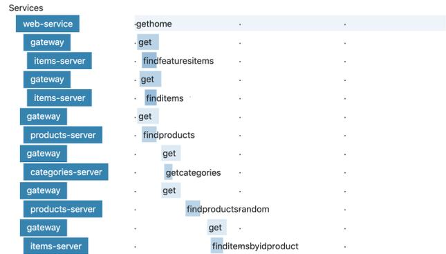
Figure 5: Gantt chart of a request loading the homepage of E-Shopper
