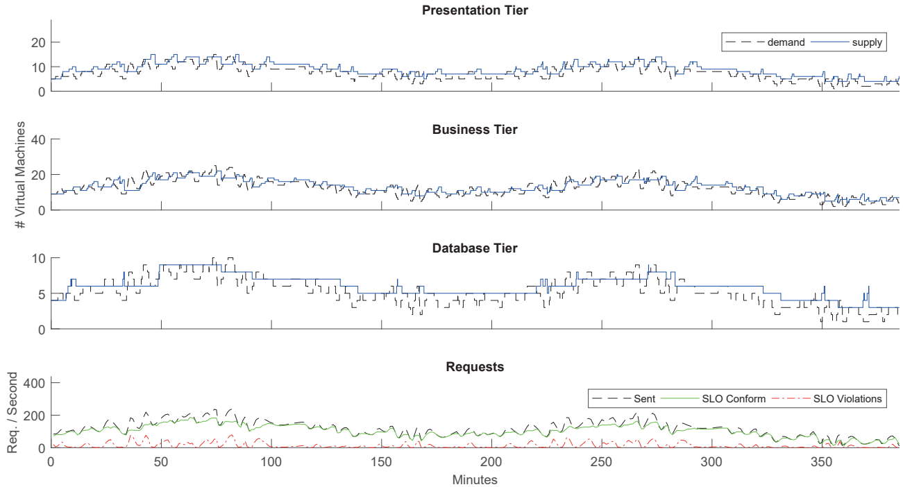
Figure 5: Scaling behavior of React without FOX on the BibSonomy trace with Amazon EC2 cost model.
