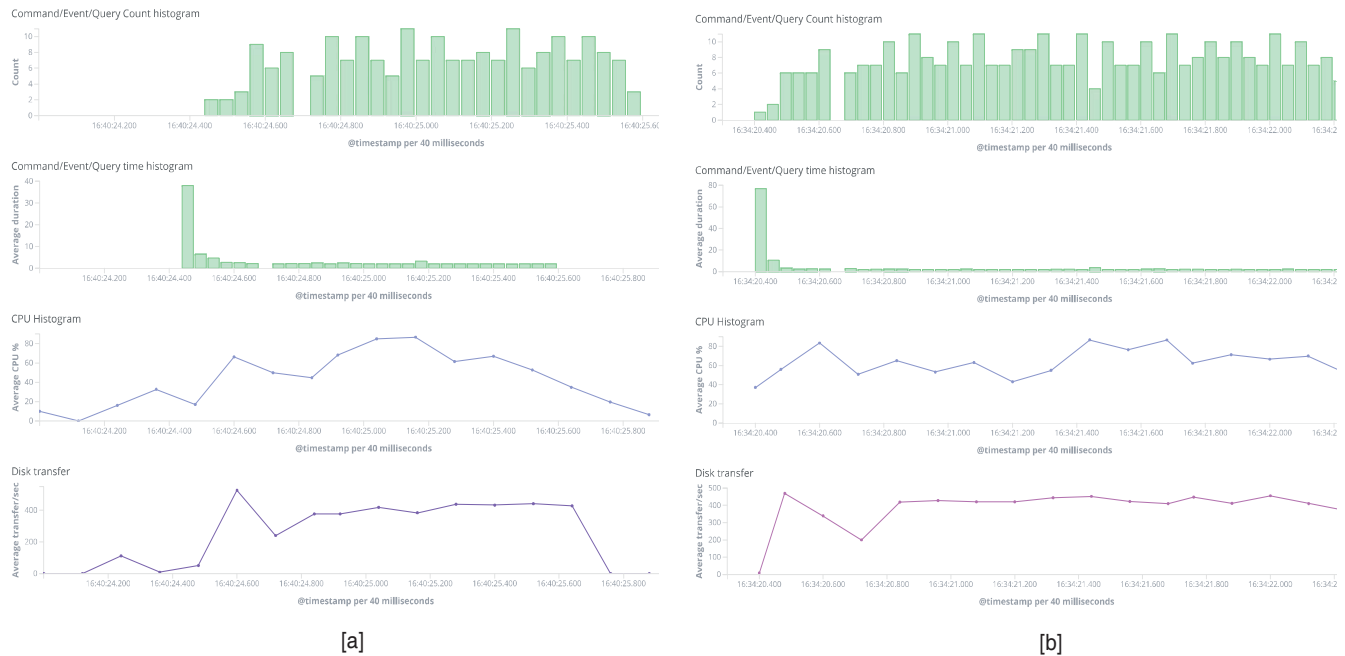
FIGURE 7. KIBANA DASHBOARD FOR WORKLOAD SIMULATION FOR AN ORGANIZATION IN [A] CL5 AND [B] CL18. WE IN PARTICULAR NOTE THE LONGER RAMP-UP AND STEADY DROP IN CPU AND DISK TRANSFER AT THE END OF THE TEST OF THE ORGANIZATION IN CL5.
