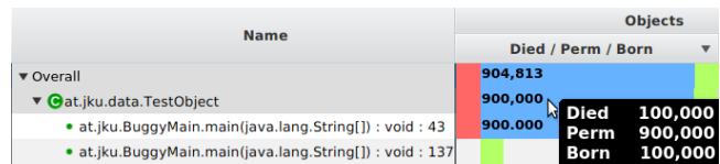
Figure 14: Heap diff of the buggy stack implementation.
