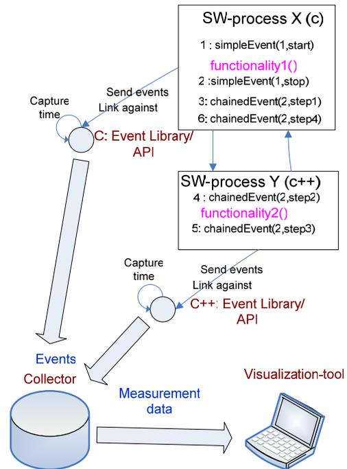
Figure 1. System architecture of the tool.
