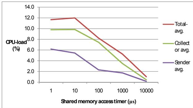
**Figure 8. CPU-processing caused by the tool as a function of shared memory access. 'Total avg.' is the average of total CPU-processing. Average CPU-consumption caused by the Collector, and Sender (EventLibrary) is also described.**
