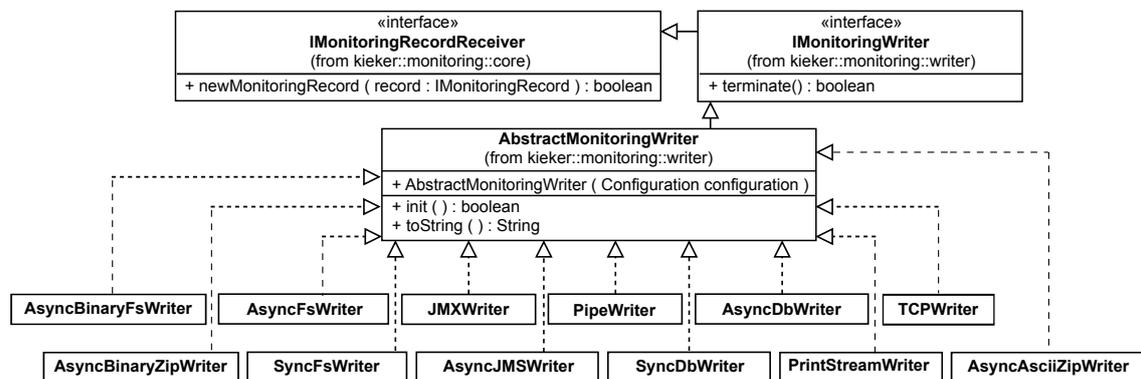
Figure 3.4: Interface `IMonitoringWriter` and the implementing classes
