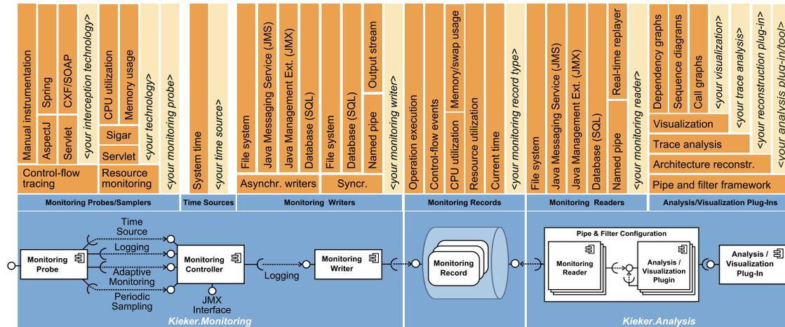
Figure 1.3: Kieker framework components and extension points for custom components
