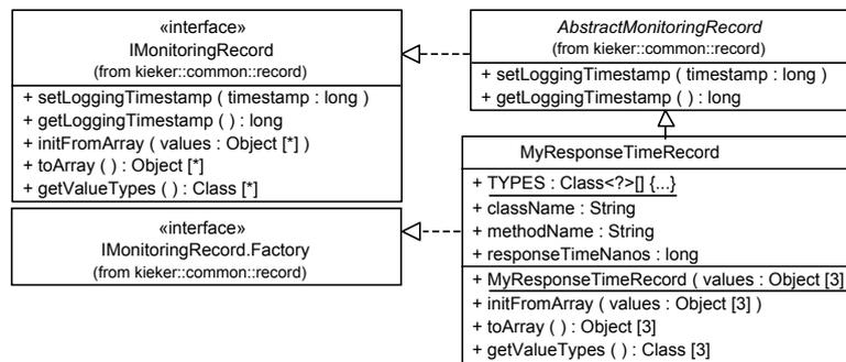
Figure 3.3: Class diagram with the `IMonitoringRecord` and `IMonitoringRecord.Factory` interfaces, the abstract class `AbstractMonitoringRecord`, and a custom monitoring record type `MyResponseTimeRecord`
