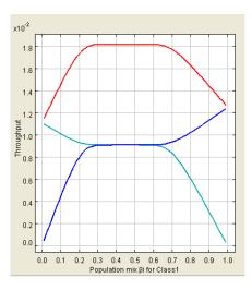
Figure 5: *Throughput* of the system (red curve) and per-class (blue curve for class 1 and light blue for class 2), as a function of the fraction of requests of the two classes in execution.
