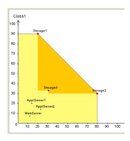
Figure 4: Visual representation of the service demands and identification of the bottlenecks as resources that lie on the convex hull.
