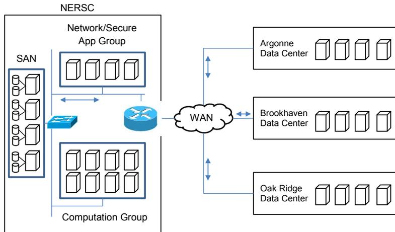
Figure 1-1: Data transfer and synchronization between data centers. This is an example from the Department of Energy’s (DOE’s) Magellan cloud data centers that are interconnected by multiple 100 Gbps links of the DOE’s Advanced Network Initiative.
