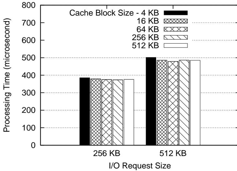
Figure 5-10: Processing time with various cache block sizes.
