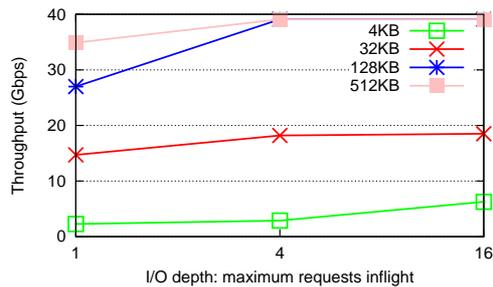
Figure 3-6: RDMA asynchronous performance in 40 Gbps Ethernet.
