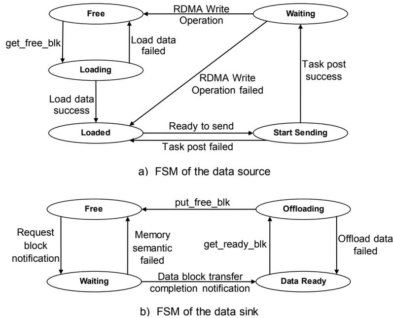
Figure 4-2: User payload block's finite state machine.
