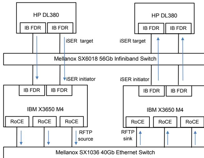
Figure 6-4: RDMA-based end-to-end system connectivity in LAN.
