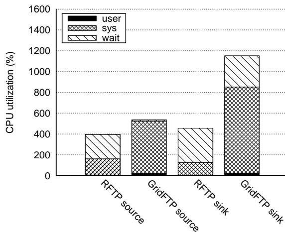
Figure 6-9: CPU utilization breakdown for RFTP and GridFTP.
