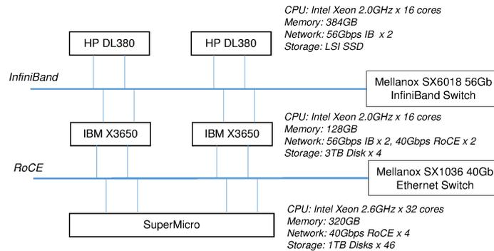
Figure 3-5: Testbed connectivity.
