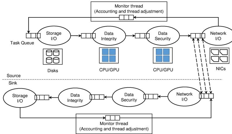
Figure 3-2: End-to-end asynchronous software architecture.
