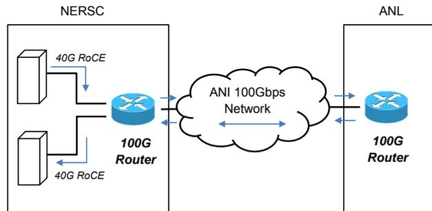
Figure 6-5: The DOE's ANI 40 Gbps RoCE WAN between NERSC and ANL. This 4000-mile link is a loopback network from NERSC to ANL and then back to NERSC. The RTT of the link is about 95 milliseconds.
