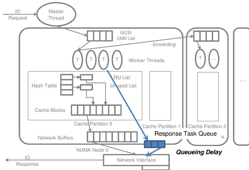
Figure 5-13: Queuing delay in iSCSI target system. We monitor the delay in the network buffer queue at user space.
