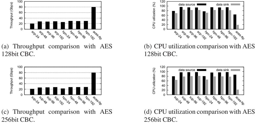
Figure 3-7: Performance comparison among OpenSSH-SCP, HPN-SSH, and ACES-FTP. The numbers in X-axis is the parallel processes launched during experiments.
