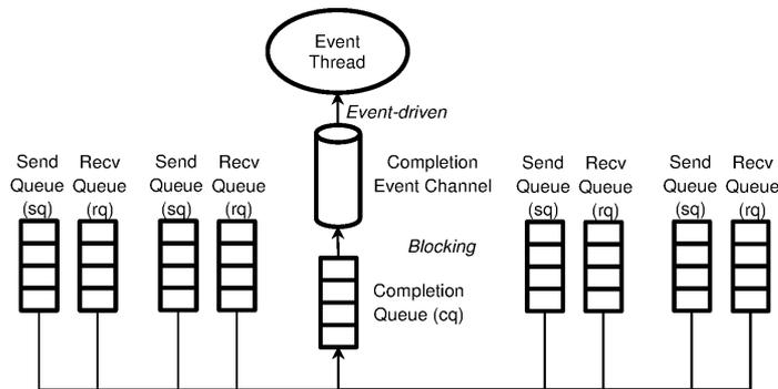
Figure 5-7: Centralized processing for RDMA network events.
